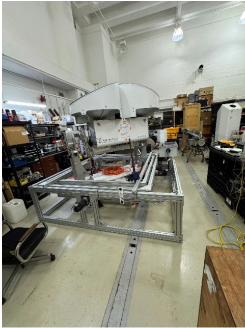
Figure 8: While the radar was under construction by RPG, Research Engineer Scott Coppersmith designed and constructed a motion stabilizing platform for the Ka-W band radar. Upon delivery of the radar, the platform was adjusted to be fully compatible with the radar. The working miniaturized demonstrator (Figure 6) and simulator (Figure 7) helped the full-scale development.
