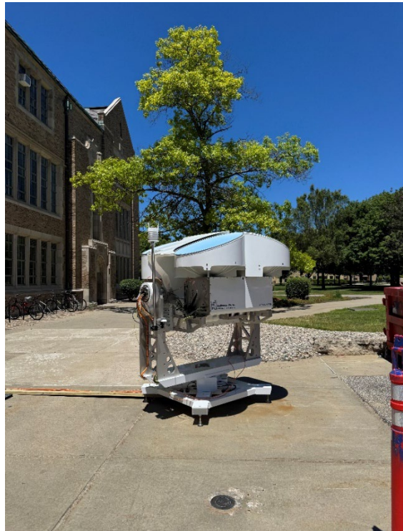
Figure 1: The Ka-W Combo (both FMCW) system being assembled and tested after arrival in UND. This off-the-shelf system enhances radar [remote sensing] research capabilities by conjoining the existing RPG W-band radar with a new Ka-band radar (both FMCW) on a common scanning platform. The radar attracted a lot of attention when it was placed outside, with many people stopping to ask about the equipment and its purpose. The second picture shows the radar set up outside on a cloud-free day for calibration against the sky.
