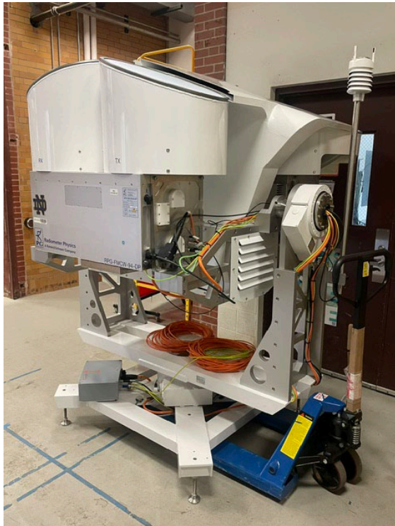
Figure 1: The Ka-W Combo (both FMCW) system being assembled and tested after arrival in UND. This off-the-shelf system enhances radar [remote sensing] research capabilities by conjoining the existing RPG W-band radar with a new Ka-band radar (both FMCW) on a common scanning platform. The radar attracted a lot of attention when it was placed outside, with many people stopping to ask about the equipment and its purpose. The second picture shows the radar set up outside on a cloud-free day for calibration against the sky.
